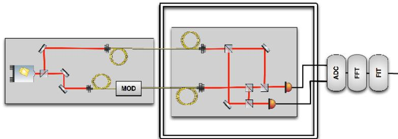
Schematic of the setup with the modulation bench (left), the Mach-Zehnder interferometer inside the vacuum chamber (middle) and the post-processing taking place in the FPGA (right).
